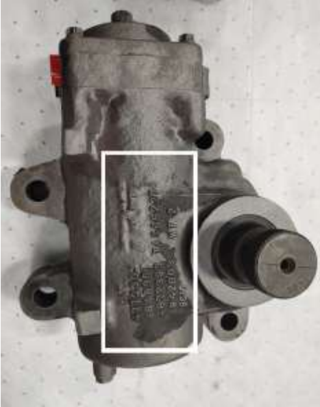
TRW LOGO AND SERIAL NUMBERS STAMPED INTO HOUSING
